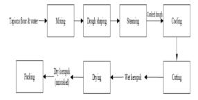
Figure 1. Flow chart of Cracker Production
